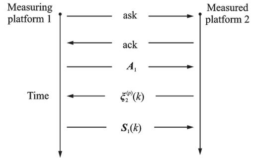
Fig.3 Mutual communication progress between the measuring and measured platform for the source location information generating
