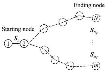
Fig.4 Illustration of all the communication topologies suitable for UKF-DCL
