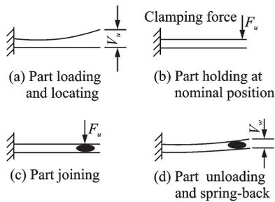
Fig.1 Compliant part assembly
