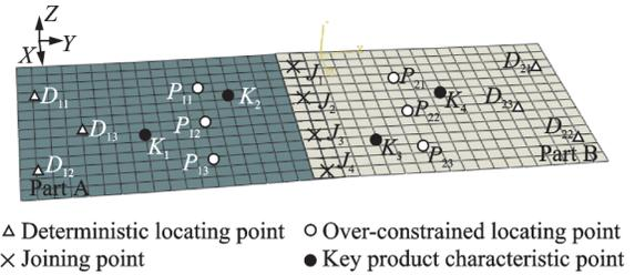
Fig.8 FEA model of sheet metal assembly
