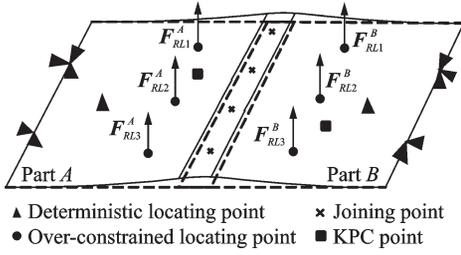
Fig.7 Clamping release at the over-constrained points
