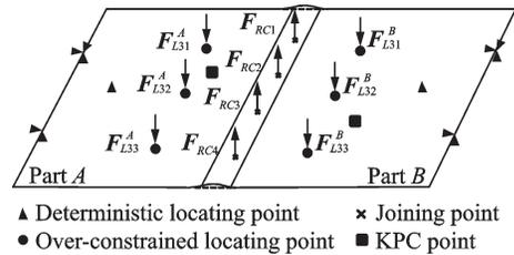
Fig.6 Clamping release at the joining points
