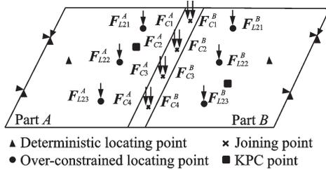
Fig.5 Applied clamping force
