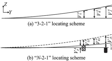
Fig.4 Locating errors of Part A
