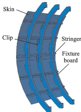
Fig.9 A typical 3D model of fuselage panel
