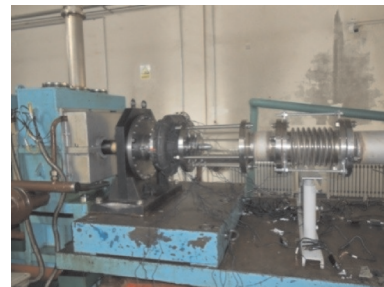
Fig.3 Redesigned pipe assembly
