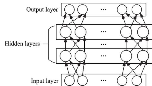
Fig.2 Structure of DNN
