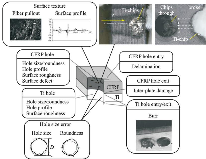
Fig.6 Hole quality features of FRP/metal stacks<sup>[8,30]</sup>
