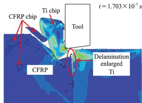
Fig.9 Chip formation process under the Ti→CFRP cutting sequence<sup>[43]</sup>
