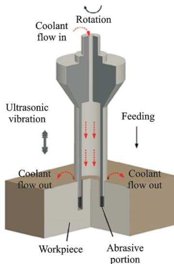
Fig.14 Illustration of ultrasonic assisted drilling<sup>[70]</sup>
