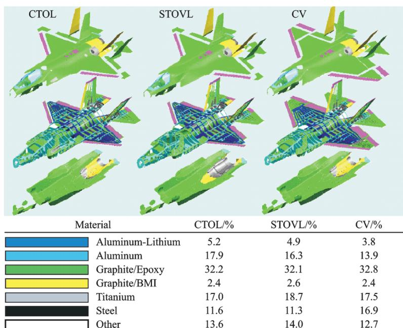
Fig.1 Schematic diagram of F-35 materials<sup>[3]</sup>
