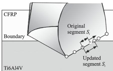
Fig.2 Schematic of drilling bi-material interface<sup>[21]</sup>
