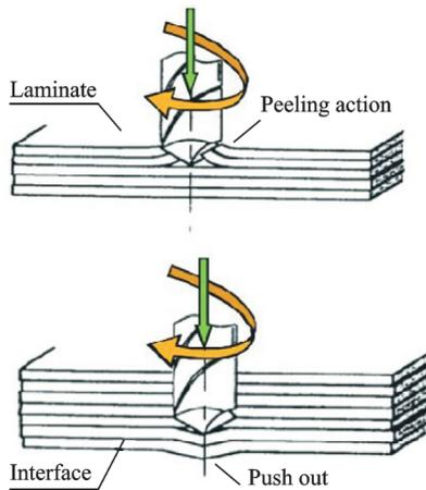
Fig.7 Delamination at the entry and exit<sup>[32]</sup>
