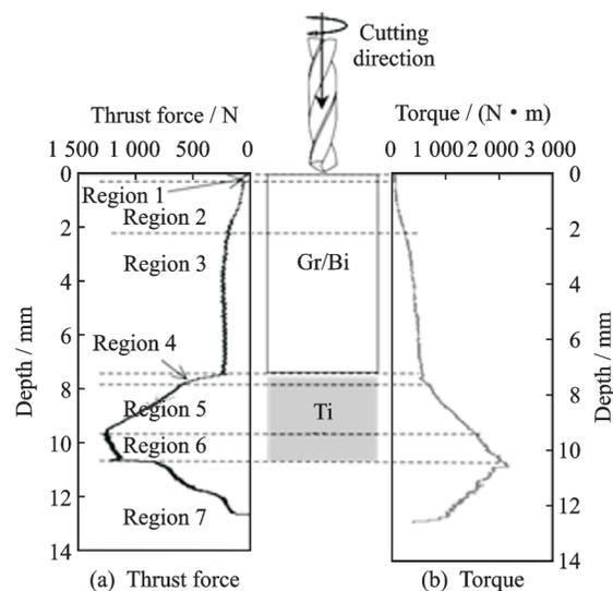
Fig.4 Typical cutting forces versus depths<sup>[23]</sup>
