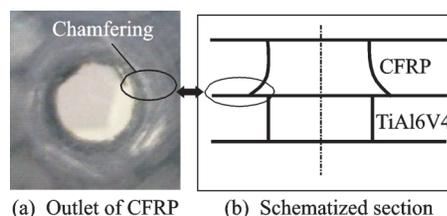
Fig.11 Microscope photograph of outlet of CFRP and schematized section of stacks after chamfering<sup>[46]</sup>
