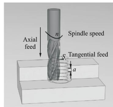
Fig.13 Schematic of helical milling process<sup>[69]</sup>
