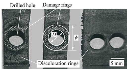
Fig.5 CFRP damage region at the CFRP/Ti interface<sup>[23]</sup>
