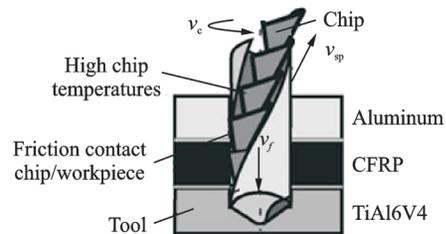
Fig.3 Chip removal problems in drilling FRP/metal stacks<sup>[22]</sup>
