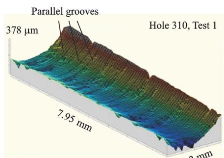
Fig.10 Topographic maps for the CFRP hole<sup>[6]</sup>
