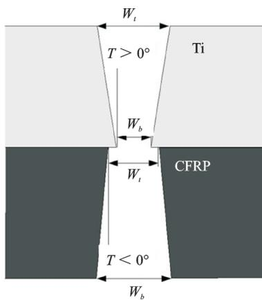
Fig.15 Example of kerf profile<sup>[79]</sup>
