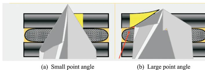
Fig.12 Effect of point angle on delamination<sup>[16]</sup>
