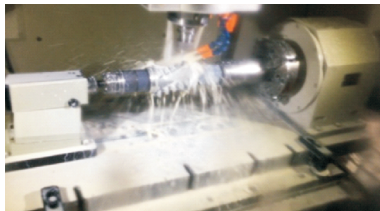
(a) Hob machining process
