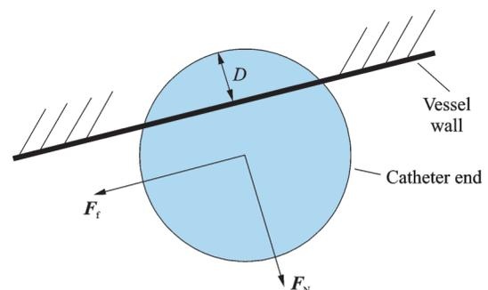
Fig.6 Feedback force calculating model
