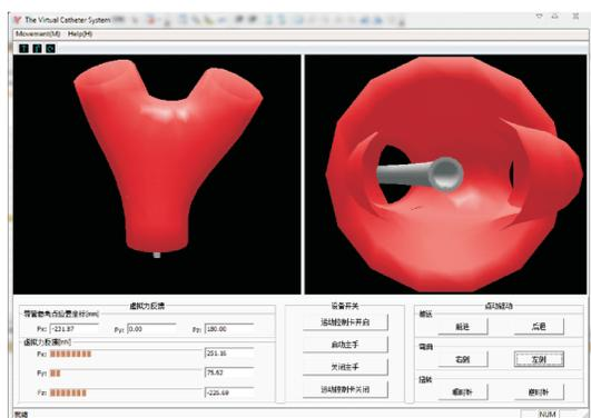
Fig.13 User interface of the virtual system
