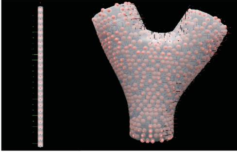
Fig.10 Skeleton filling of catheter and vessel
