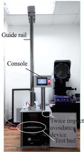
Fig.2 Impact testing machine
