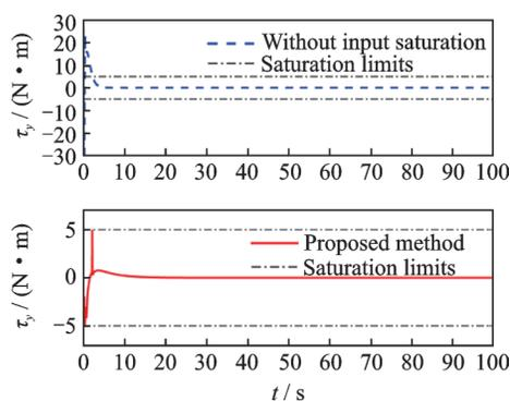
Fig.11 Control torque  $\tau_y$
