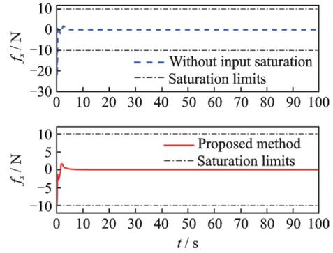
Fig.7 Control force  $f_x$
