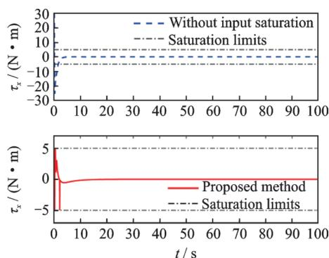
Fig.10 Control torque  $\tau_x$
