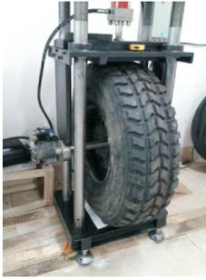
Fig.6 Tire characteristic test rig
