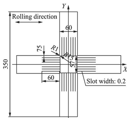
(a) Dimensions of cruciform specimen after optimized
