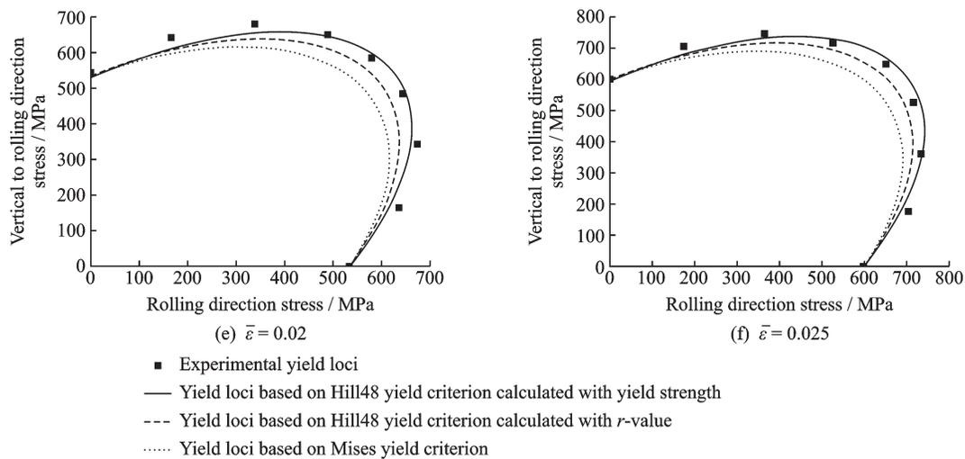
Fig. 4 Comparison between theoretical and experimental yield loci under different plastic strain
