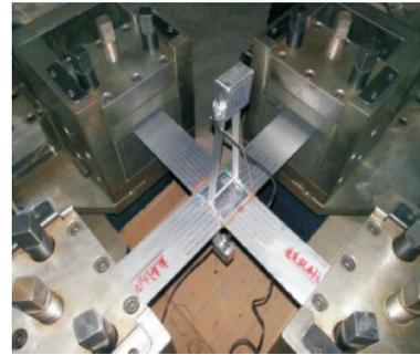
Fig.2 Establishment of the biaxial tensile test system
