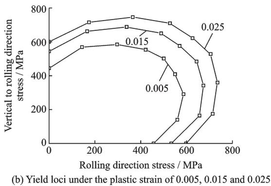
Fig.3 Yield loci under different plastic strain
