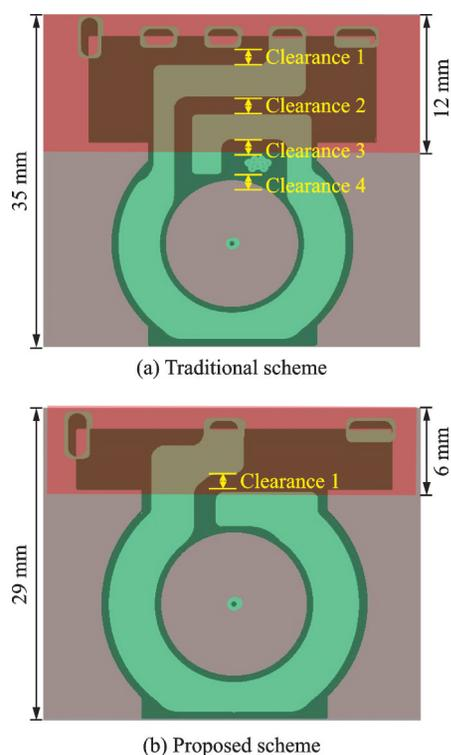
Fig.4 Comparison of PCB footprint
