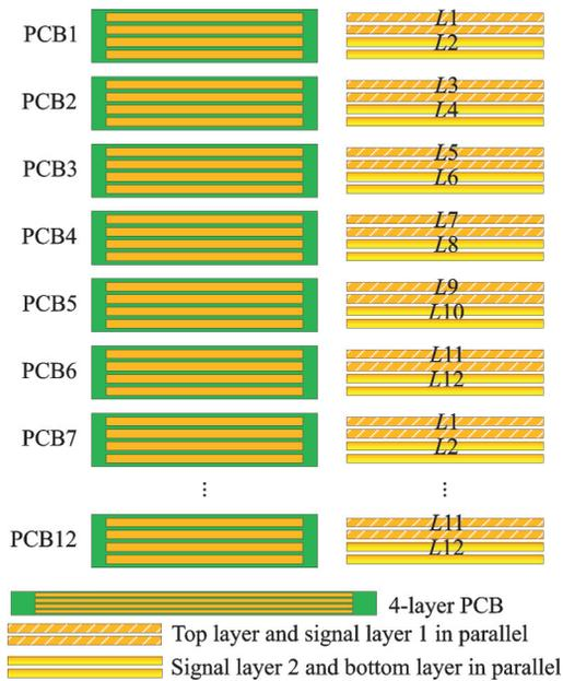
Fig.5 Winding arrangement of the proposed inductor
