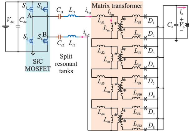
Fig.1 LLC converter with split resonant tanks
