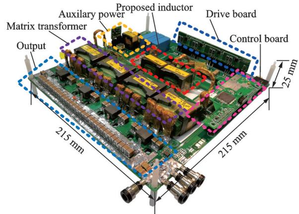
Fig. 7 Photo of prototype
