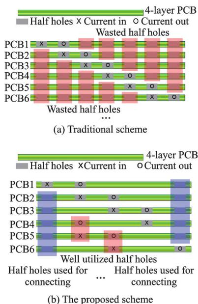
Fig.3 Comparison of winding connecting schemes
