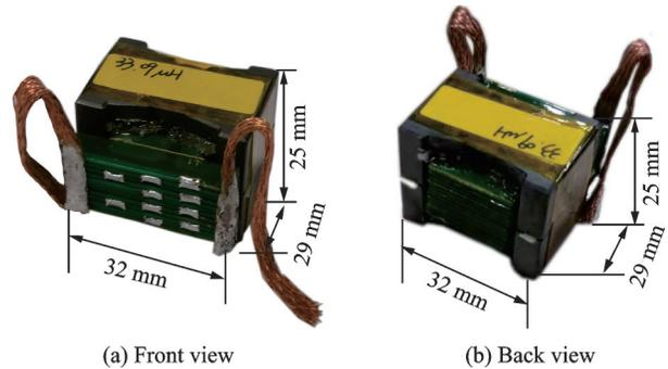
Fig. 8 Photos of resonant inductor
