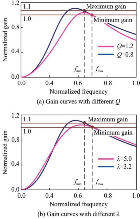
Fig.2 Gain curve of LLC converter
