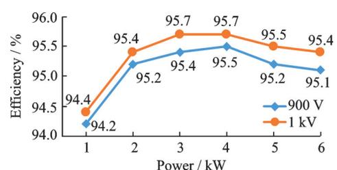
Fig.12 Efficiency curves under close-loop condition
