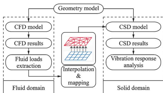
Fig. 8 Simulation procedure of one-way coupling problem
