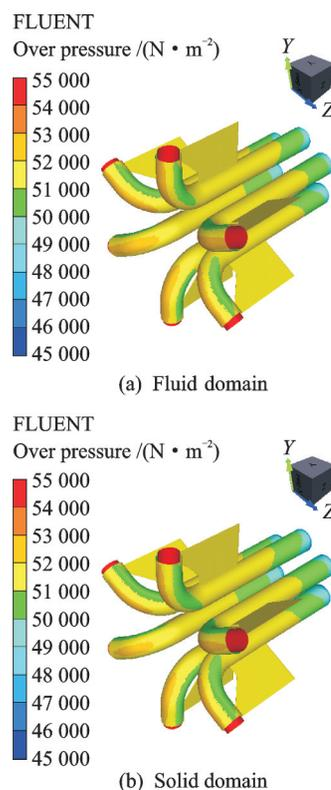
Fig. 9 Pressure contour of fluid-solid coupling field
