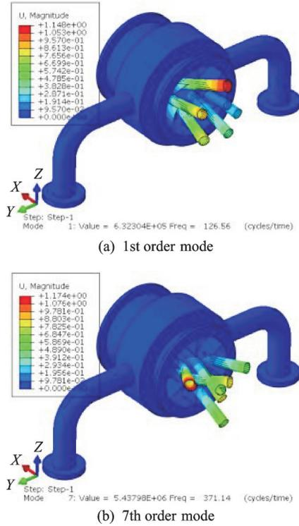
Fig.2 Mode shapes of ejector suction chamber
