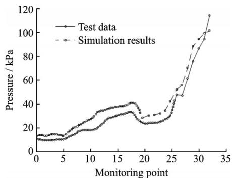
Fig.13 Static pressure distribution of ejector fluid field
