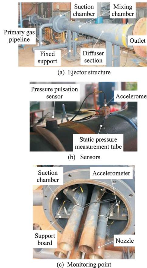
Fig.12 Vibration test platform of ejector structure
