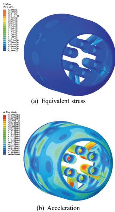
Fig.10 Transient response contour of ejector structural vibration
