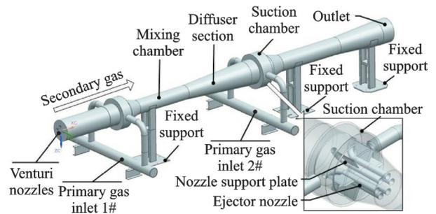
Fig.1 Composition of ejector structure
