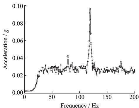
Fig.15 Acceleration test results of support plate
