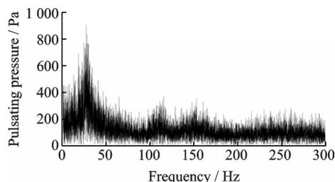
Fig.14 Test results of ejector pulse pressure
