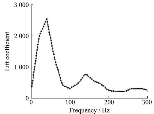
Fig.7 Frequency spectrum curve of lift coefficient in ejector
