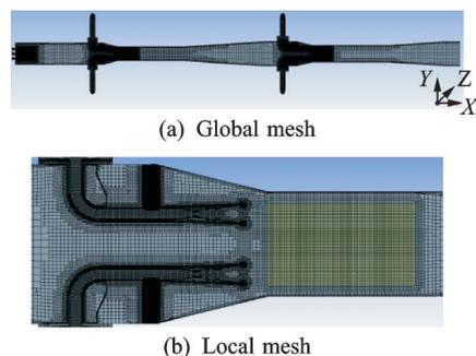
Fig.3 Fluid grid of ejector inner fluid field
