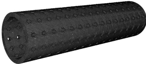
Fig.7 Geometry and finite element discretization of a medical stent
