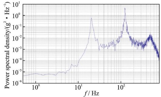
Fig.5 PSD curve of beam's end
