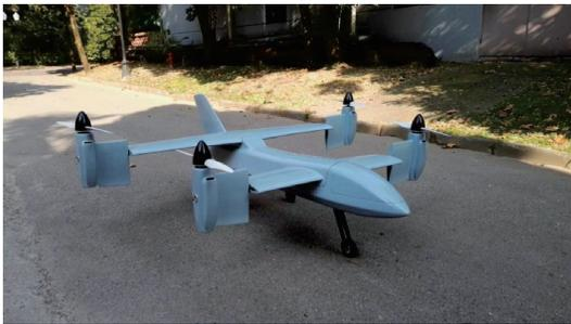
Fig.1 Tilt quad rotor with tilt-wing
