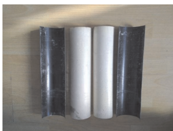
(b) Peeling surface between the outer layer and the core layer after the failure of the specimen
