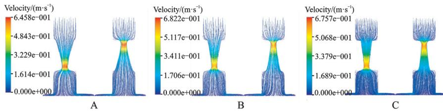
Fig.4 Velocity streamline in the suction stroke
