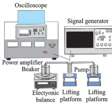
Fig.8 Experimental schematic of flow rate measurement
