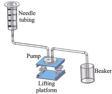
Fig.9 Experimental schematic diagram of flow resistance measurement
