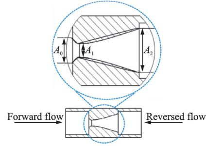
Fig.3 Sectional view of the streamlined flow tube
