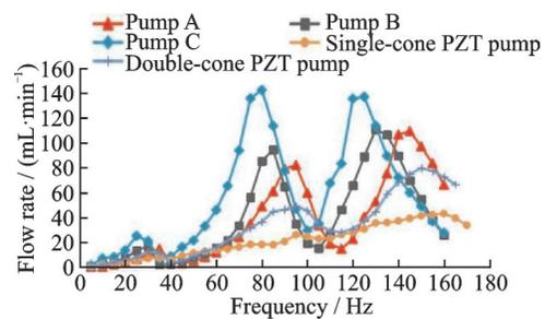
Fig.10 Flow rate comparison of white blood and deionized water in each pump
