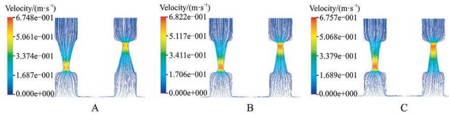
Fig.5 Velocity streamline in the exhaust stroke
