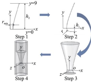
Fig.1 Flow tube design process
