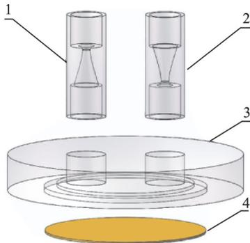
1—Streamlined flow tube A; 2—Streamlined flow tube B; 3—Pump body; 4—PZT vibrator
