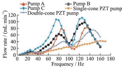
Fig.11 Experimental flow rate results of deionized water
