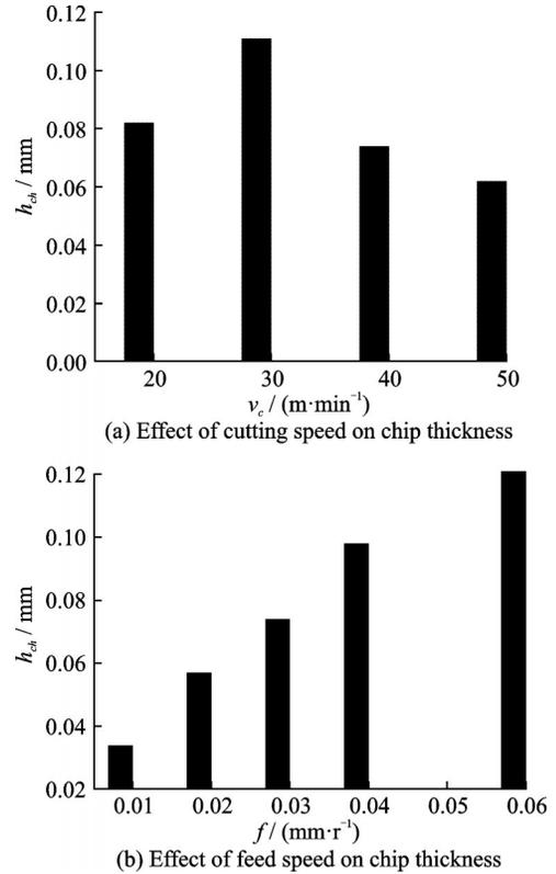
Fig.12 Effect of cutting parameters on chip thickness
