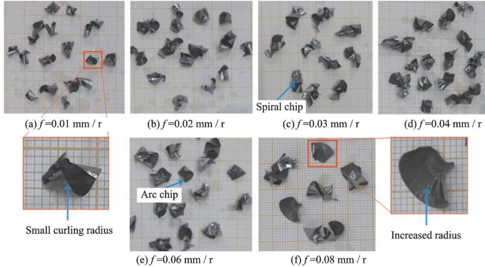
Fig.11 Effect of feed on chip deformation
