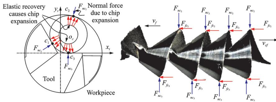
Fig.7 Normal and frictional forces acting on spiral chip due to elastic recovery
