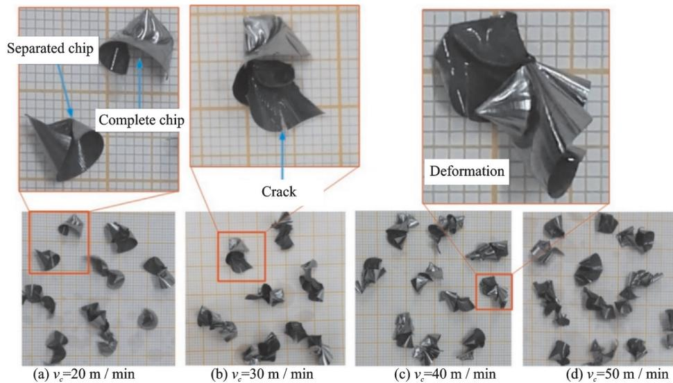
Fig.10 Effect of cutting speed on chip deformation
