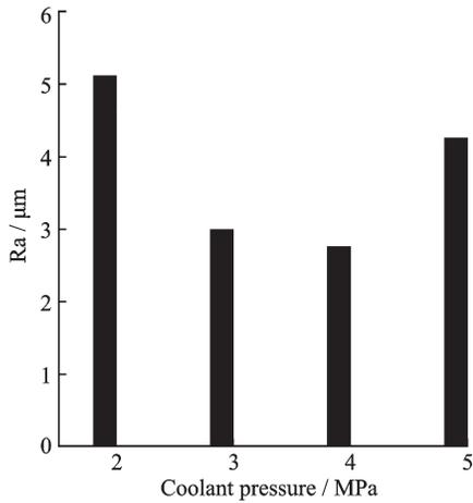
Fig.15 Relationship between coolant pressure and roughness
