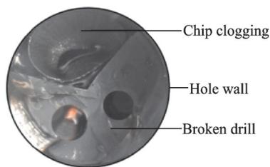
Fig.1 Broken drill due to chip clogging
