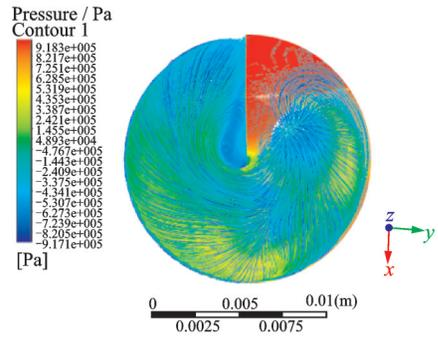
(a) Simulation diagram of vortex near the cutting edge
