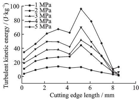
Fig.18 Turbulent kinetic energy near the edge of rake face
