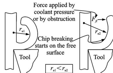
Fig.6 Increase in up-curl radius due to coolant pressure leading to chip breaking
