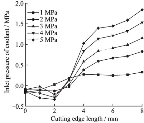
Fig.17 Coolant pressure near the cutting edge
