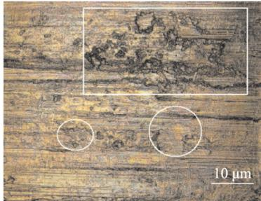
Fig.2 Micro scratches on machined surface
