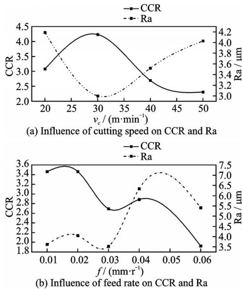
Fig.13 Influence on chip compressibility (CCR) and roughness
