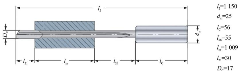
Fig.9  $\phi 17$ mm standard gun drill (unit: mm)
