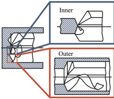
Fig.3 Chip forming process of inner and outer edges
