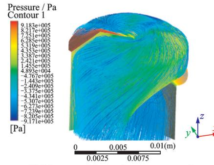
(b) Diagram of the coolant pressure at the cutting edges
