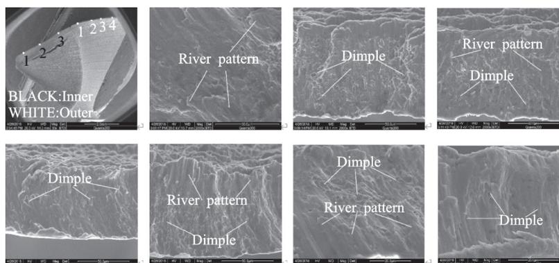
Fig.8 Electron microscopy of chip fractur
