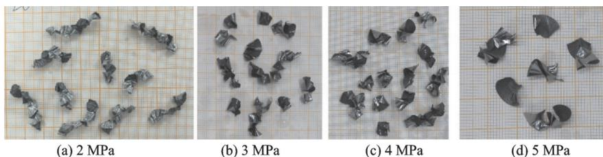
Fig.14 Effect of coolant pressure on chip morphology
