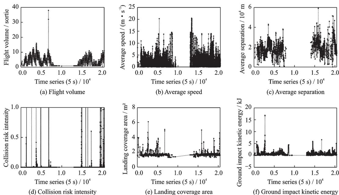
Fig.4 Change curves of UAV flight risk assessment index with time series
