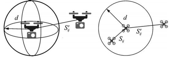
Fig.2 Schematic diagram for calculating the UAV collision risk intensity index
