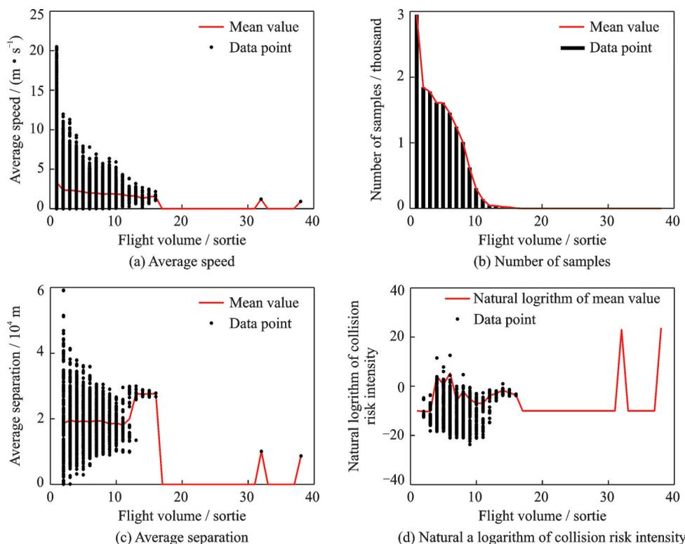
Fig.5 Correlation between UAV flight risk indexes and flight volume
