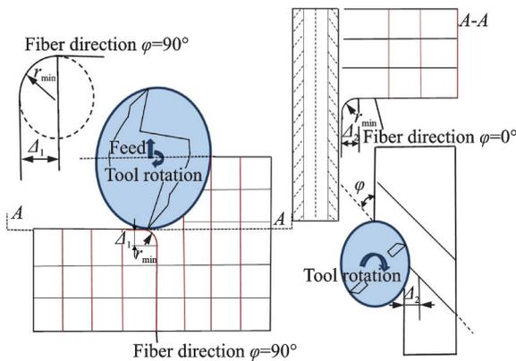
Fig.8 Bending of fibers in laminate and vertical planes
