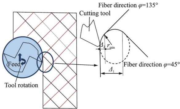
Fig.7 Bending of fibers in laminate plane at different fiber directions
