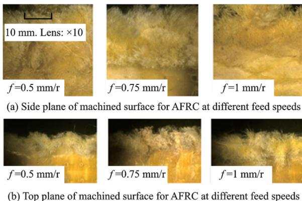
Fig.2 Delamination defects for AFRC for machining directions at  $0^\circ$
