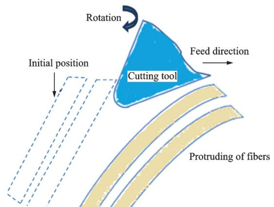
Fig.4 Schematic of the development of delamination
