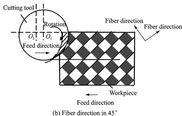
Fig.6 Explanation of feed rate effects on delamination defect
