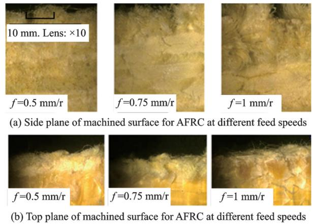
Fig.3 Delamination defects for AFRC for machining directions at  $45^\circ$
