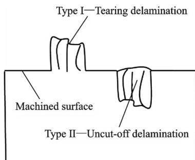
Fig.5 Types of delamination for machined surface
