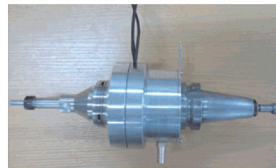
Fig.8 Prototype of giant magnetostrictive ultrasonic vibration device for progressive sheet forming
