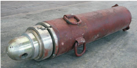
Fig.1 Hydraulic support column
