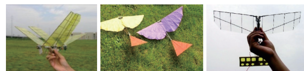
(a) NWPU-PY-6 (b) NWPU-PY-7 (c) NWPU-PY-8 Fig.4 Bionic flapping-wing micro air vehicles of NWPU-PY-6, NWPU-PY-7 and NWPU-PY-8
