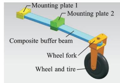
Fig.1 Sketch map of unmanned aircraft composite landing gear
