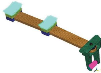
Fig.3 Finite element model of composite landing gear
