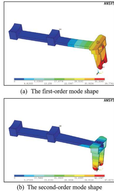
Fig.5 Mode shapes of composite landing gear
