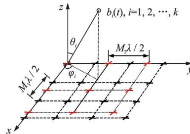
Fig.1 PS-CPA configuration with  $M_1 = 3$  and  $M_2 = 4$
