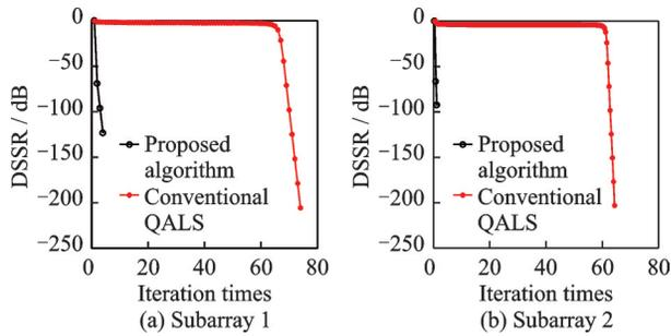
Fig.2 Convergence comparison of different algorithms
