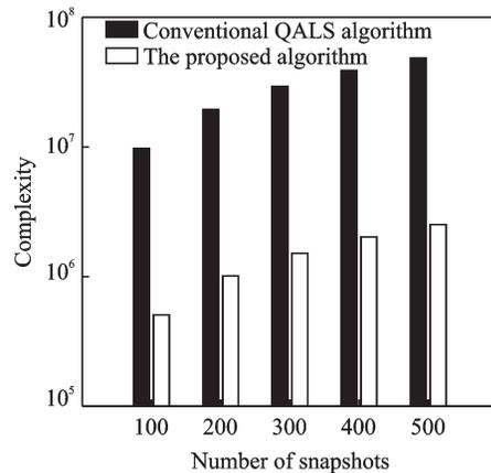
Fig.4 Complexity comparison of different snapshots between the proposed algorithm and the conventional QALS algorithm
