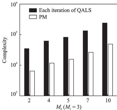
Fig.3 Complexity comparison between PM and each iteration of QALS in the PS-CPA
