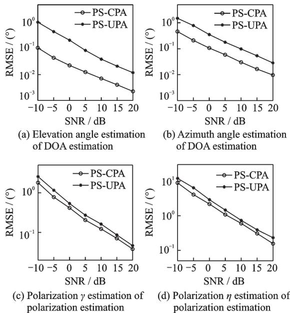
Fig.7 Parameter estimation performance of different arrays
