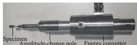
Fig.2 Terminal components of ultrasonic fatigue testing machine
