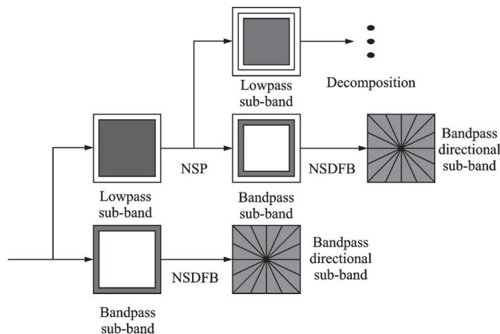
Fig.1 Decomposed structure of NSCT
