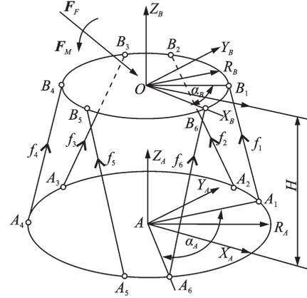
Fig.1 Statics model of Stewart-type force sensor
