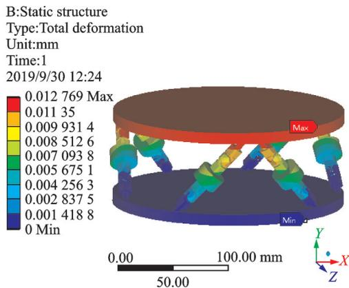
Fig.5 Total deformation of sensor in Condition 1
