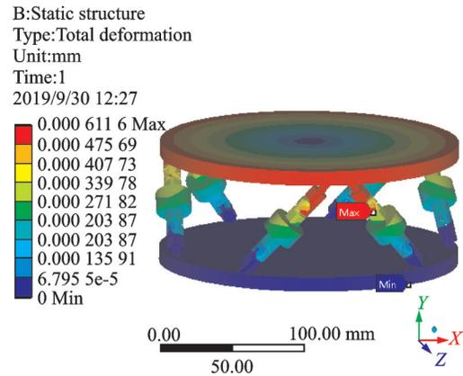
Fig.8 Total deformation of sensor in Condition 4
