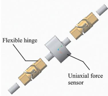
Fig.4 Explosion diagram of the component.
