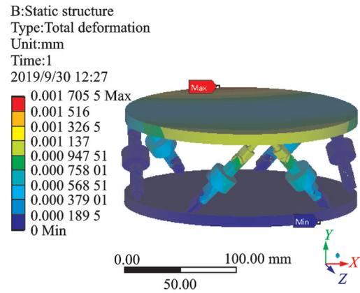
Fig.7 Total deformation of sensor in Condition 3
