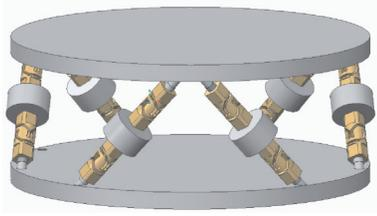
Fig.3 Stewart platform-based force/torque sensor
