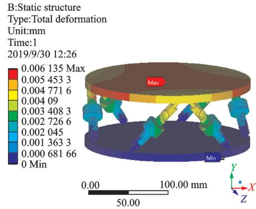
Fig.6 Total deformation of sensor in Condition 2
