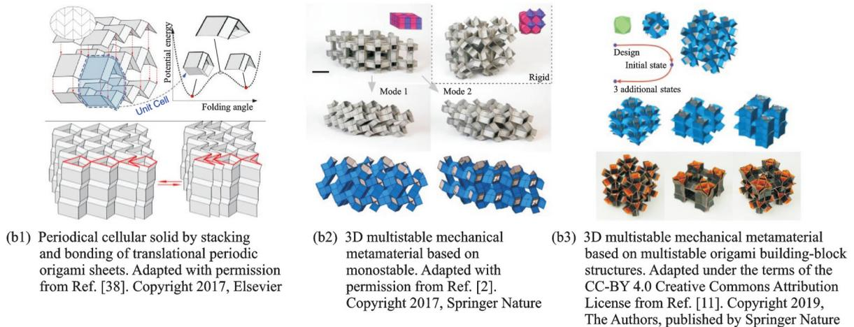
(b) Multistable metamaterials with more complex geometric configurations
