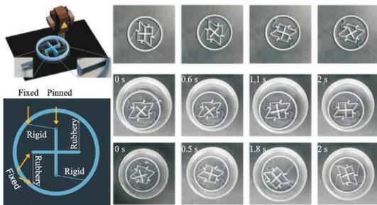
(b1) Thermal actuator of a quadristable structure. Adapted with permission from Ref.[47]. Copyright 2019, Wiley-VCH
