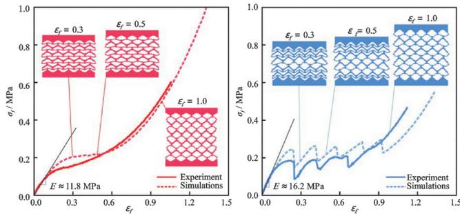
(a1) Tunable stress-strain curves. Adapted with permission from Ref. [18]. Copyright 2015, Wiley-VCH
