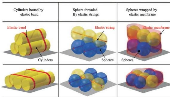
(a4) Multistable mechanical metamaterial which is self-locked by frictional force. Adapted with permission from Ref. [35]. Copyright 2019, Wiley-VCH
