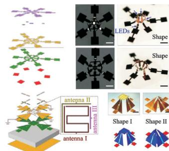
(a2) Morphable 3D optoelectronic and electromagnetic devices. Adapted with permission from Ref.[5]. Copyright 2018, Springer Nature
