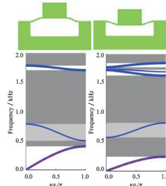
(c3) Dispersion relations for bistable unit cells for the initial and deformed stable configurations. Adapted with permission from Ref.[42]. Copyright 2017, Elsevier
