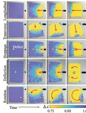
(c2) Propagations of 2D transition wave, including wave pinning, wave deflection and rotation. Adapted with permission from Ref.[15]. Copyright 2020, National Academy of Sciences
