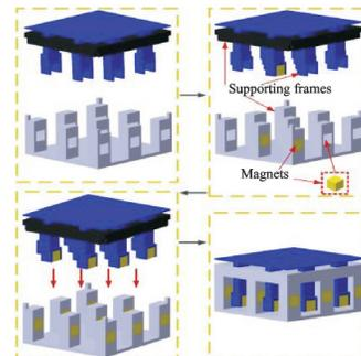
(a5) Multistable mechanical metamaterial which is self-locked by magnetic force. Adapted with permission from Ref. [36]. Copyright 2019, Elsevier
