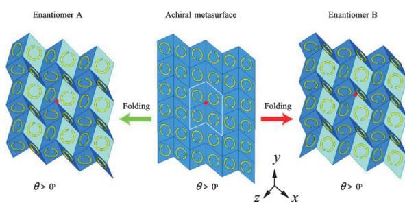
(a1) Reconfigurable electromagnetic metamaterials with chiral responses. Adapted with permission from Ref.[16]. Copyright 2017, Wiley-VCH
