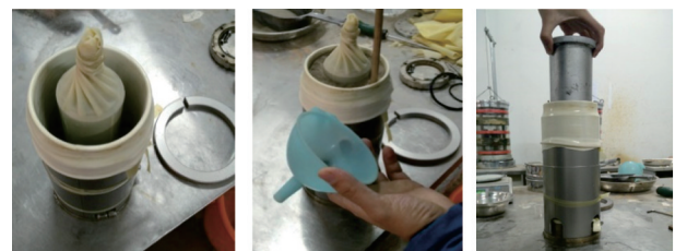
(a) Fixing of inner and outer membranes
