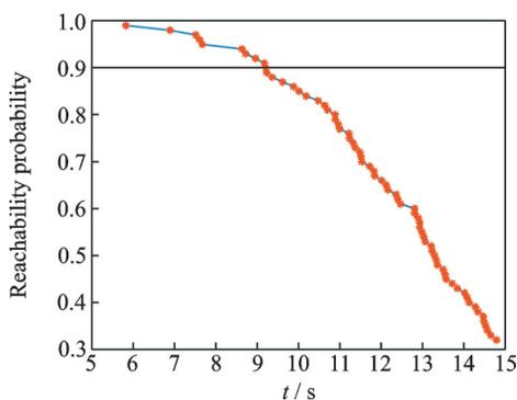
Fig.13 Distribution diagram of turbulent reachability probability under the level IV turbulence
