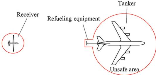
Fig.4 Collision range of the receiver and the tanker
