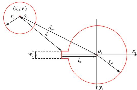
Fig.5 Collision detection of the aerial refueling system
