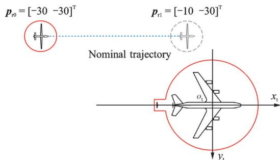
Fig.7 Nominal trajectory of the receiver
