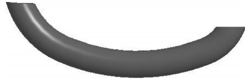
Fig.7 Three-dimensional model of hydraulic flow channel based on B-spline curve
