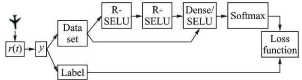
Fig.3 Structure diagram of overall training network
