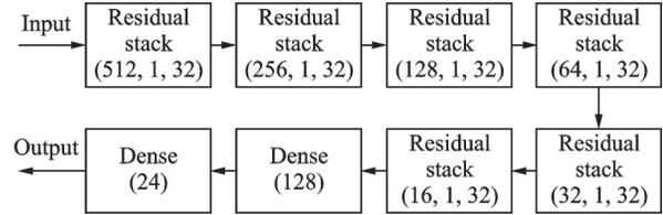
Fig.2 Structure of ResNet network
