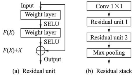
Fig.1 Residual block structure
