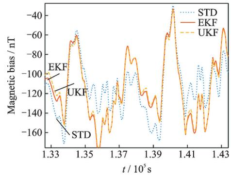
Fig.4 Magnetic biases of EKF and UKF
