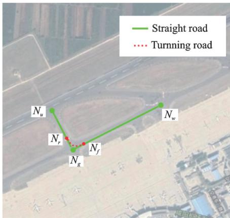
Fig.2 Aircraft turning section taxiing process
