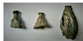
(e) Photo of experimental result: Solidification of metal melt at front end of melt delivery tube ( p = 4.5 MPa, 18Ni300)
