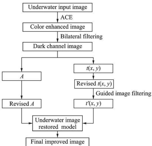
Fig.1 Flow chart of the proposed algorithm
