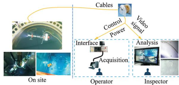
Fig.2 Schematic of underwater NPP visual inspection
