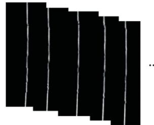
(b) Laser stripes projected onto the cup
