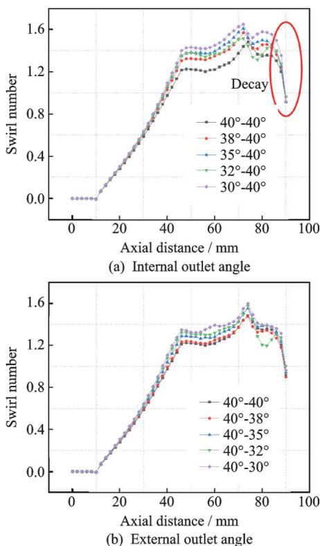
Fig.5 Swirl numbers of axial cyclone tubes
