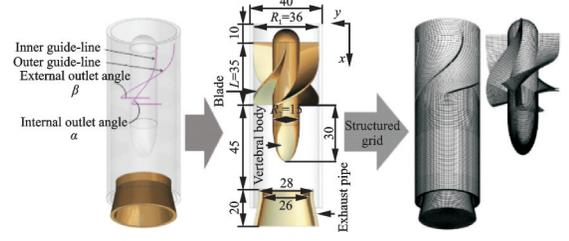
Fig.1 Definition of cyclone tube parameters and structural grid
