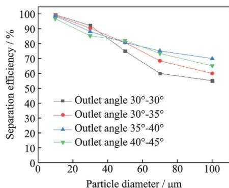
Fig.10 Separation efficiency of guide vane axial flow cyclone tube with different blade parameters
