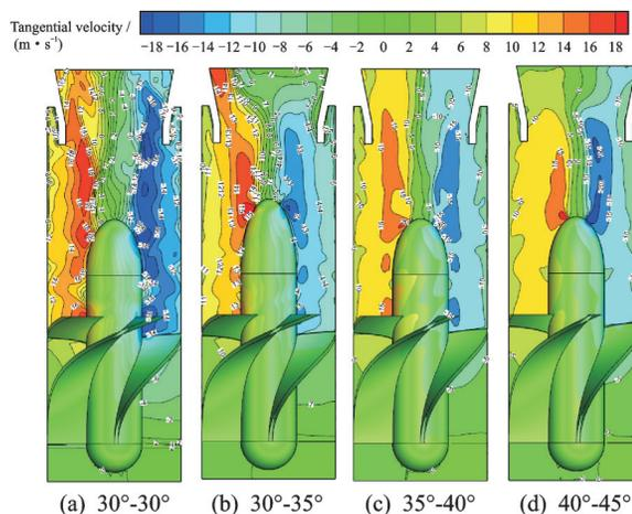
Fig.6 Nephograms of tangential velocity with different internal-external outlet angles
