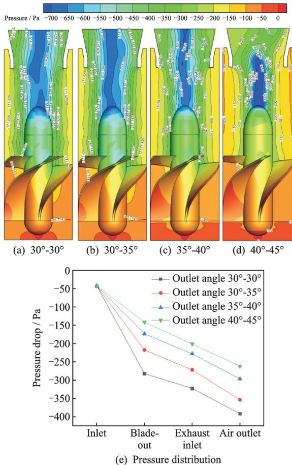
Fig.8 Pressure with different internal and external outlet angles
