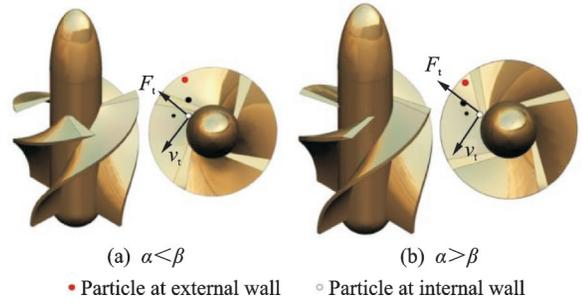
Fig.3 Force condition of particles
