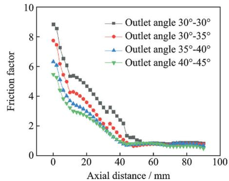
Fig.9 Friction factor of the guide vane axial flow cyclone tube with different blade parameters
