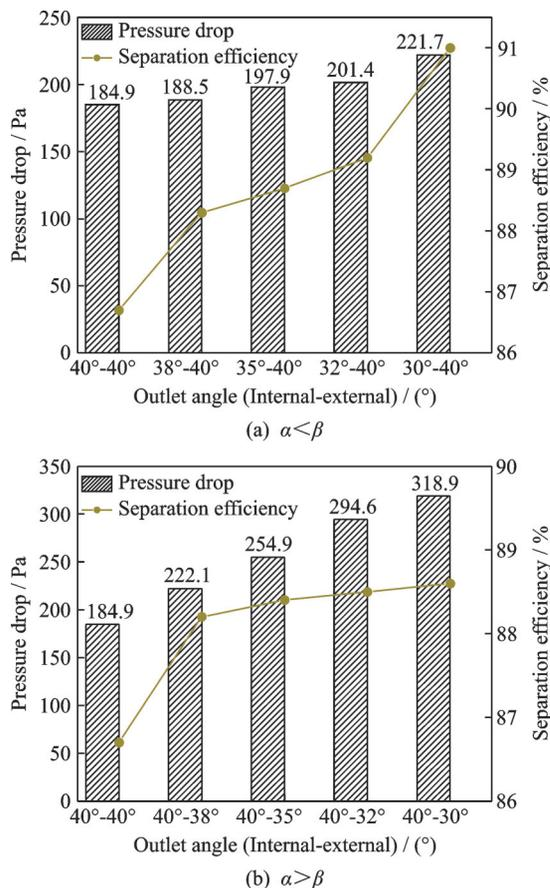
Fig.4 Effect of two outlet angles on cyclone performance
