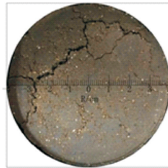
Fig.6 Cracks on the upper surface of the soil column after ten dry-wet cycles [17]
