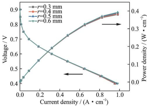
Fig.10 Polarization curve and power curve of HT-PEMFCs with different baffle radii
