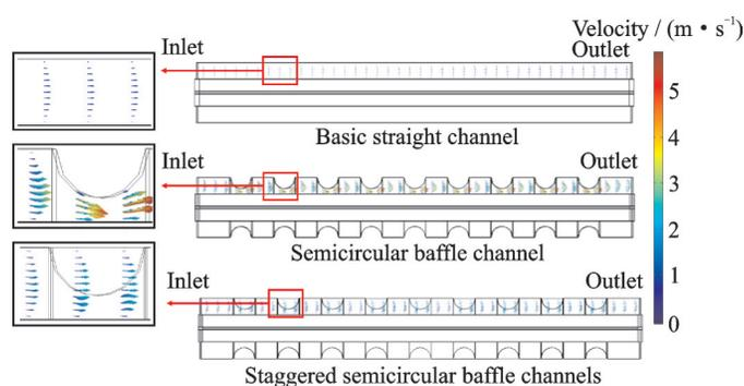
Fig.16 Velocity vector in cathode gas channel ( $V_{\text{cell}} = 0.4 \text{ V}$ ,  $r = 0.5 \text{ mm}$ ,  $N = 9$ )
