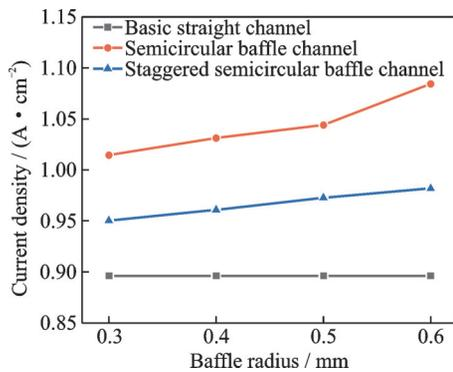
Fig.13 Influence of baffle radius on current density ( $V_{\text{cell}} = 0.4 \text{ V}$ ,  $r = 0.5 \text{ mm}$ ,  $N = 9$ )
