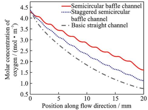
Fig.8 Oxygen molar concentration in three flow channels along the flow direction in GDL-CL plane
