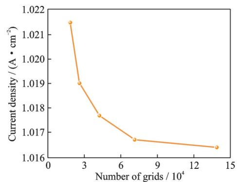
Fig.5 Grid independence verification diagram.
