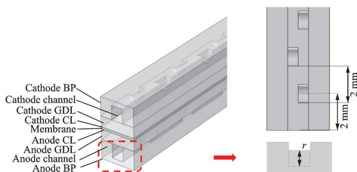
Fig.2 Geometric diagram of PEMFC with staggered semicircular baffle channel
