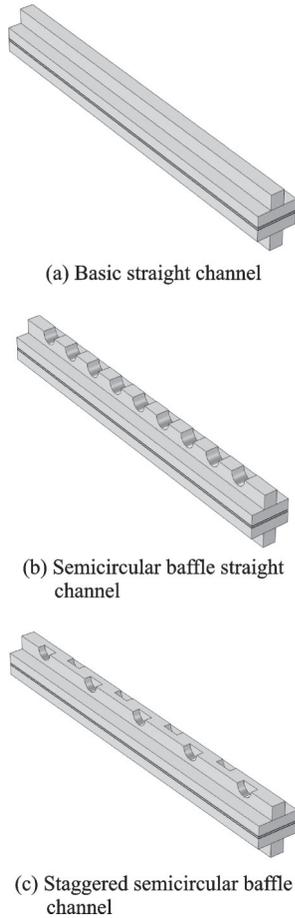
Fig.3 Computational domain of PEMFCs with different channels
