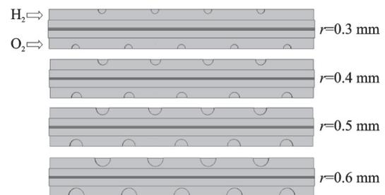
Fig.9 Schematic diagram of different baffle radii in the bipolar plate channel
