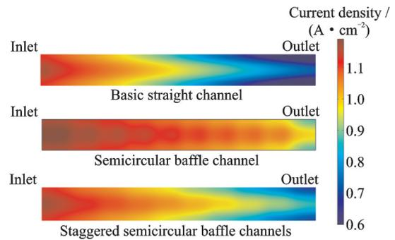
Fig.15 Distribution of current density at the middle plane of membrane ( $V_{\text{cell}} = 0.4 \text{ V}$ ,  $r = 0.6 \text{ mm}$ ,  $N = 9$ )
