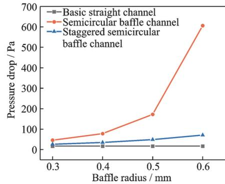
Fig.14 Influence of baffle radius on cathode pressure drop ( $V_{\text{cell}} = 0.4 \text{ V}$ ,  $r = 0.5 \text{ mm}$ ,  $N = 9$ )
