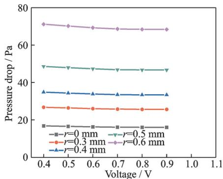
Fig.11 Pressure drop in cathode bipolar plate channel with different baffle radii
