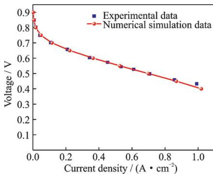
Fig.6 Comparison of simulation and experimental polarization curves of a straight-channel PEMFC
