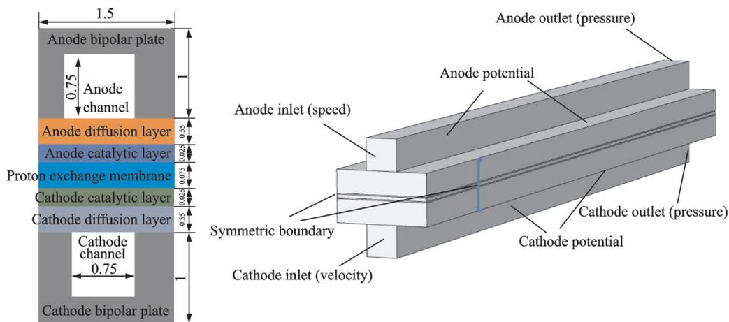
Fig.4 Basic dimensions and boundary types of the model (unit: mm)
