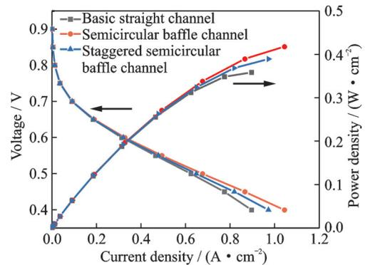
Fig.7 Polarization curve and power curve of three flow channels
