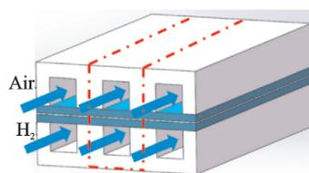
Fig.1 Position of single channel PEMFC in flow field
