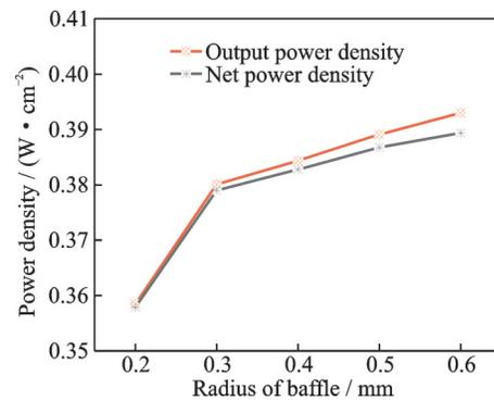
Fig.12 Comparison of output power and net power of HT-PEMFC bipolar plate channel cells with different bottom baffle radii
