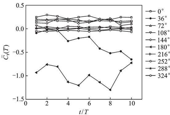
Fig.3 Cycle-by-cycle  $\bar{C}_T(T)$  curves for  $\varphi$  of  $0^\circ$ ,  $36^\circ$ ,  $72^\circ$ ,  $108^\circ$ ,  $144^\circ$ ,  $180^\circ$ ,  $216^\circ$ ,  $252^\circ$ ,  $288^\circ$  and  $324^\circ$
