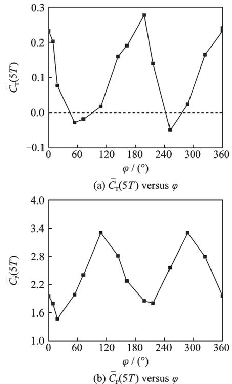
Fig.4 The mean thrust and power coefficient for  $\varphi$  of  $0^\circ$ ,  $36^\circ$ ,  $72^\circ$ ,  $108^\circ$ ,  $144^\circ$ ,  $180^\circ$ ,  $216^\circ$ ,  $252^\circ$ ,  $288^\circ$  and  $324^\circ$
