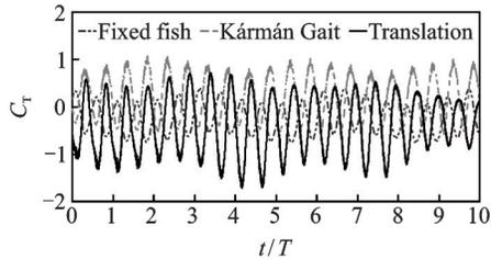
(c) Time history of  $C_T$  for the fixed fish, the Kármán gaiting fish with  $\phi$  of  $0^\circ$ , and the undulatory fish
