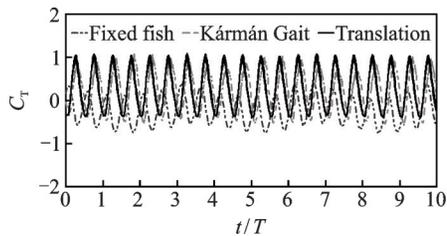
(a) Time history of  $C_T$  for the fixed fish, the Kármán gaiting fish with  $\phi$  of  $0^\circ$ , and the translating fish
