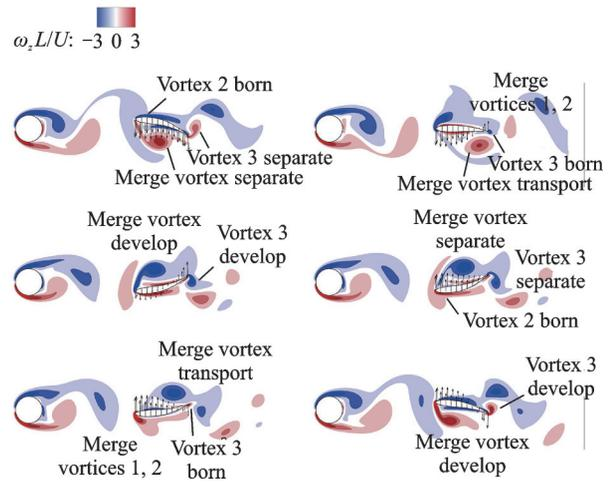
Fig.8 Instantaneous vortex distribution around the fish in one kinematic cycle for  $\phi$  of  $54^\circ$
