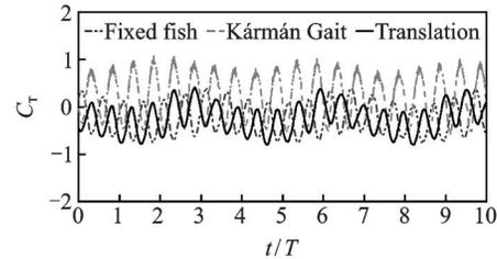
(d) Time history of  $C_T$  for the fixed fish, the Kármán gaiting fish with  $\phi$  of  $0^\circ$ , and the heading fish
