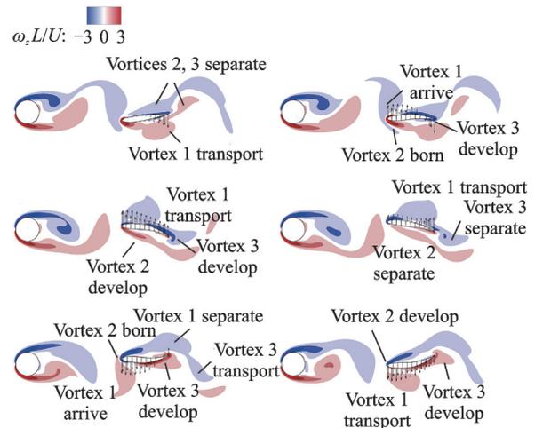
Fig.9 Instantaneous vortex distribution around the fish in one kinematic cycle for  $\phi$  of  $108^\circ$
