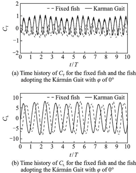
Fig.5 Time histories of  $C_T$  and  $C_L$  for the fixed fish and the fish adopting the Kármán gait with  $\varphi$  of  $0^\circ$
