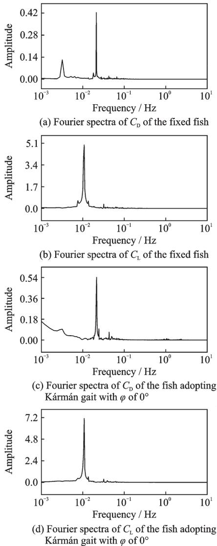
Fig.7 Fourier spectra of  $C_D$  and  $C_L$  of the fixed fish and the fish adopting the Kármán gait with  $\phi$  of  $0^\circ$
