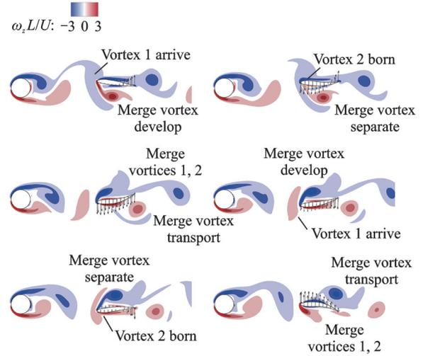
Fig.6 Instantaneous vortex distribution around the fish in one kinematic cycle for  $\varphi$  of  $0^\circ$
