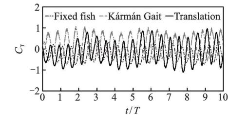
(b) Time history of  $C_T$  for the fixed fish, the Kármán gaiting fish with  $\phi$  of  $0^\circ$ , and the rotating fish
