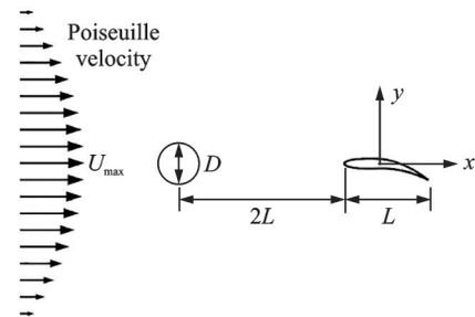
Fig.1 Flow configuration composed of a stationary cylinder and a streamlined fish
