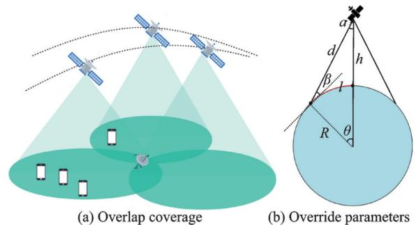
Fig.3 Communication scene and coverage model
