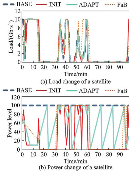
Fig.9 Single satellite change with time
