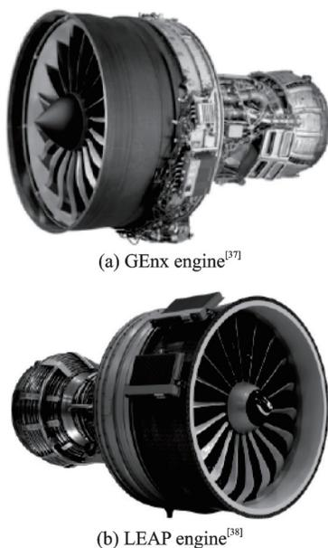
Fig.10 Aero engines adopting carbon fiber reinforced resin composite materials
