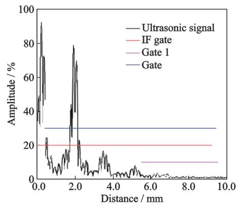
(b) Calibration by setting amplitude of the flaw echo at the distance of 1.9 mm to be close to 80%
