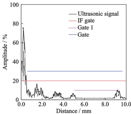
Fig.14 Comparison of echos between layers from interfaces and from internal defects
