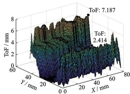
Fig.8 Three-dimensional model of internal defects
