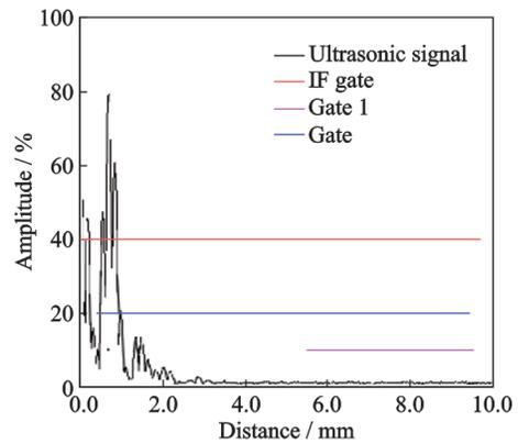
(a) Calibration by setting amplitude of the flaw echo at the distance of 0.8 mm to be close to 80%
