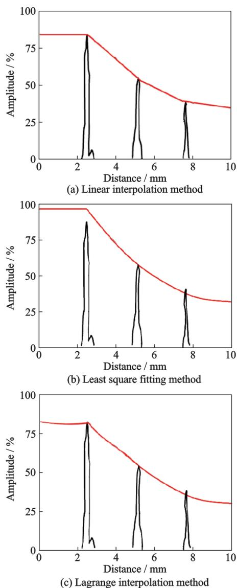
Fig.3 Bus lines of DAC constructed by using three methods
