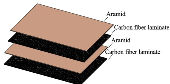
Fig.11 Typical layout of the rotor casing of aero engines
