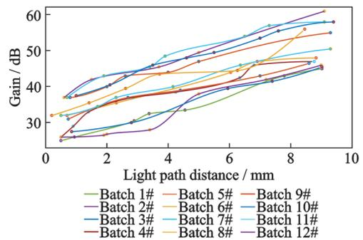
Fig.16 DAC curves of all batches
