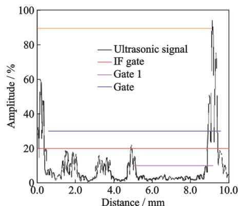
Fig.17 Comparison of echos between layers from internal defects and from interfaces
