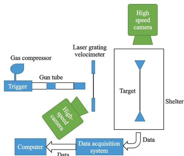
Fig.12 Schematic diagram of experiment setup
