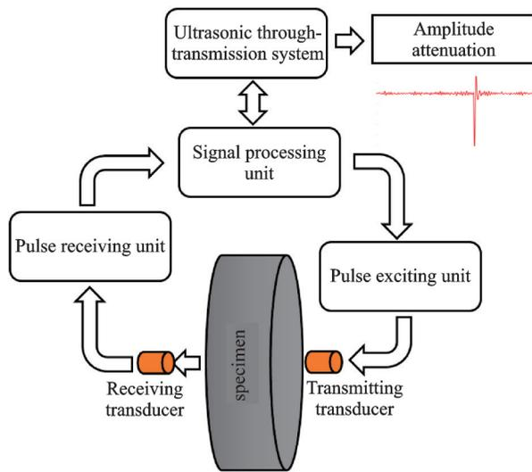
Fig.1 Schematic diagram of the ultrasonic transmission method
