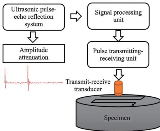
Fig.2 Schematic diagram of the ultrasonic pulse-echo method
