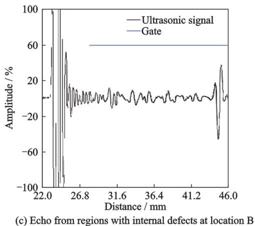
Fig.6 Experimental results of Type A pulse reflection ultrasonic testing
