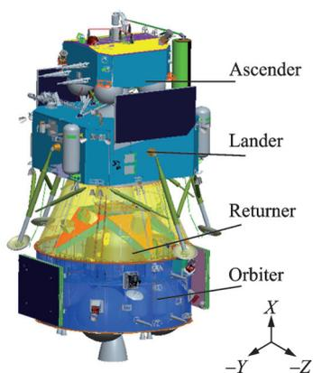
Fig.1 Overall configuration and coordinate system of Chang'e-5 explorer
