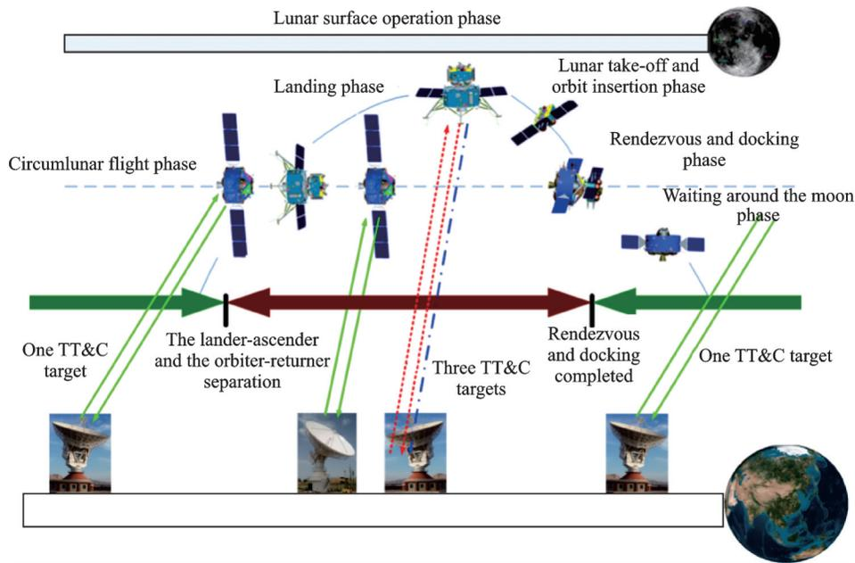
Fig.4 Diagram of multi-target TT&C requirement in X-band
