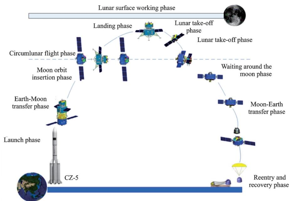
Fig.2 Schematic diagram of the whole mission flight process
