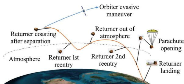
Fig.3 Schematic diagram of the reentry section
