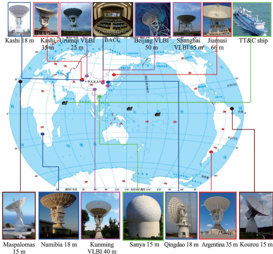
Fig.5 Layout of the TT&C network for Chang'e-5 mission
