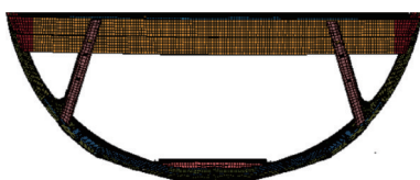
Fig.6 Maximum deformation diagram of cargo hold area impacted on water
