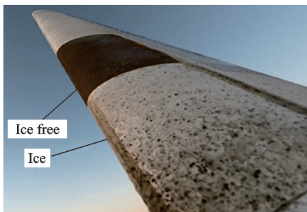
Fig.9 Photo of the flight test of the anti-icing hybrid skin
