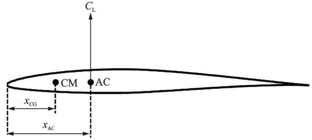
Fig.25 Airfoil aerodynamic center and CM
