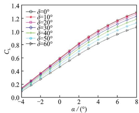
Fig.8 Lift coefficient  $C_L$  under different folding angles
