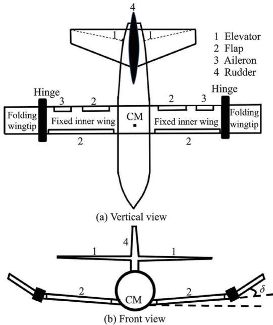
Fig.4 Geometric model of Cessna 550
