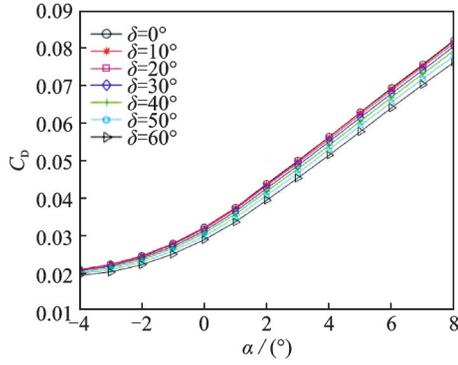
Fig.10 Drag coefficient  $C_D$  under different folding angles
