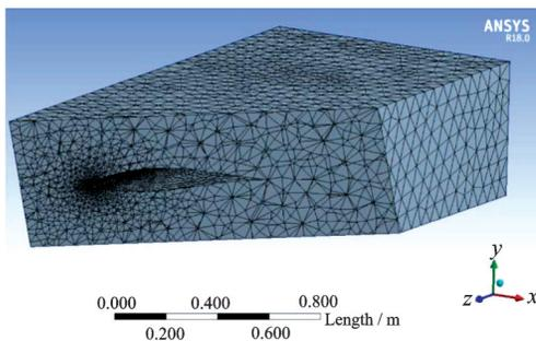
Fig.6 Aircraft wing grid model generated in Ansys
