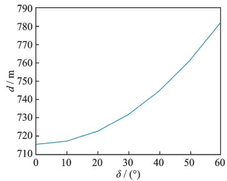
Fig.22 Landing distance under different folding angles
