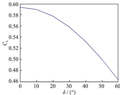
Fig.17 Liftoff lift coefficient under different folding angles
