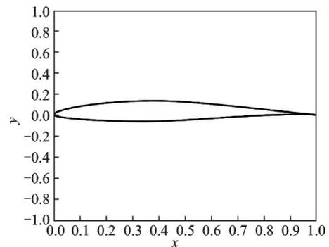
Fig.3 Airfoil of Cessna 550 aircraft
