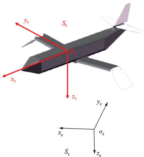
Fig.7 Coordinate axis definition
