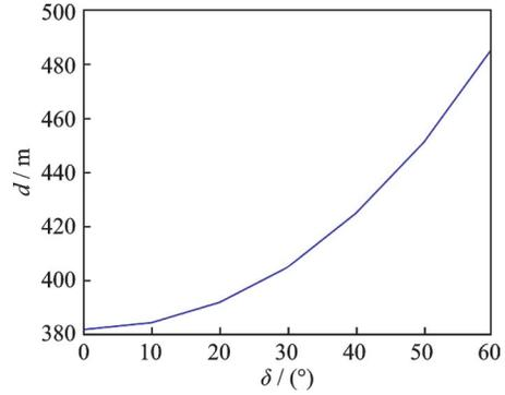
Fig.18 Taking off distance  $d$  under different folding angles
