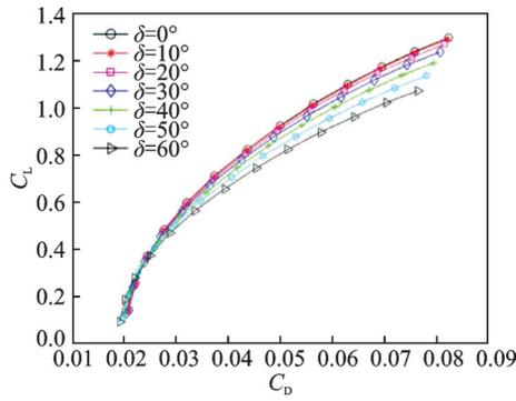
Fig.11 Polar curves under different folding angles
