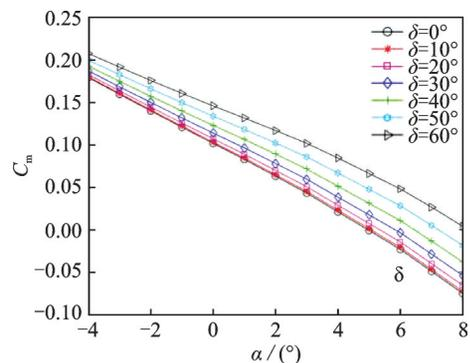
Fig.9 Pitch moment coefficient  $C_m$  under different folding angles
