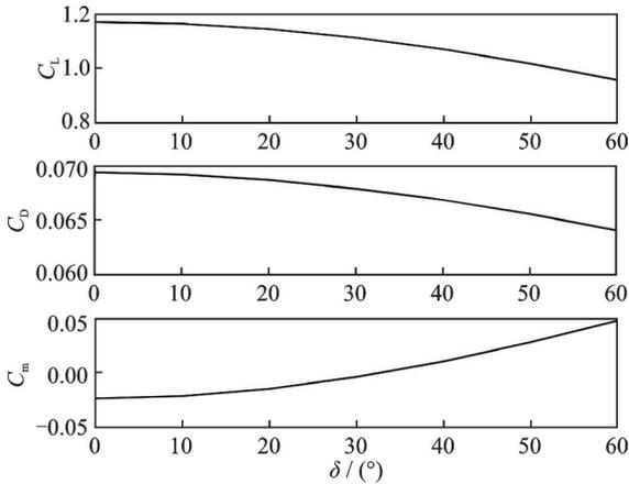
Fig.12 Aerodynamic coefficients with respect to  $\delta$  under  $\alpha = 6^\circ$
