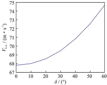
Fig.15 Liftoff velocity  $V_{L_{\text{lof}}}$  under different folding angles
