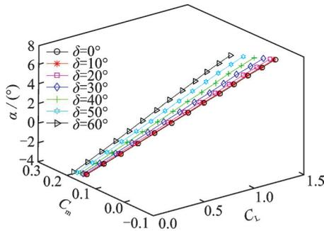
Fig.24 Longitudinal steady stability under different folding angles
