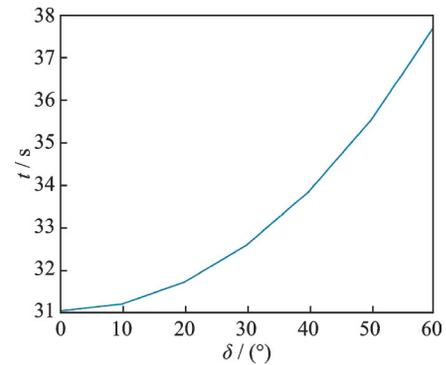
Fig.23 Landing time  $t_1$  under different folding angles
