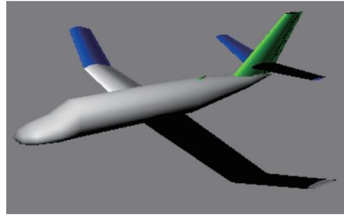
Fig.2 Cessna 550 aircraft with wing tip folding at 30°
