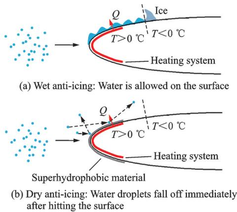
Fig.1 Principle of dry anti-icing method
