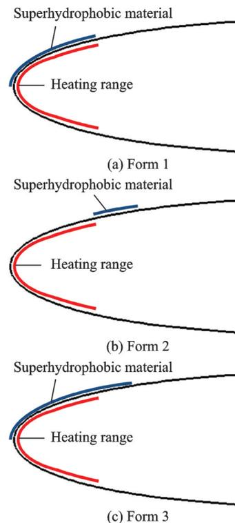
Fig.3 Layout of superhydrophobic materials
