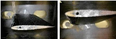
Fig.12 Anti-icing failure in Case 5
