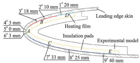
Fig.6 Electric heating and thermocouple distribution
