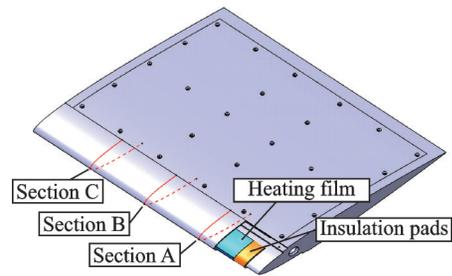
Fig.5 Experimental model and sensor sections
