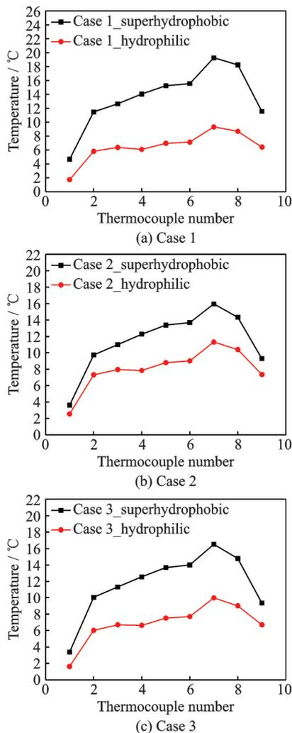
Fig.9 Surface temperature comparison of the low-energy dry anti-icing method and the traditional thermal protection method
