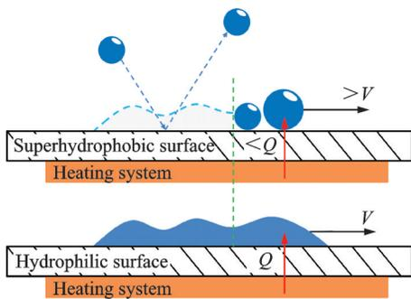
Fig.2 Principle of low-energy consumption
