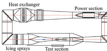
Fig.4 Structural diagram of FL-61 wind tunnel
