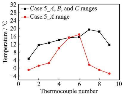
Fig.13 Surface temperature comparison between *A*, *B*, and *C* heating ranges and *A* heating range
